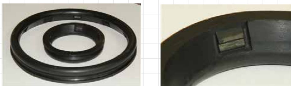
Fig. 2.10.14: Modified Gaskets with Steel Inserts
