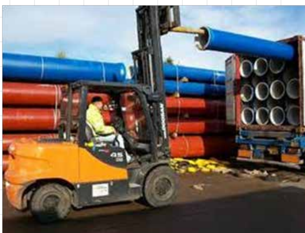
Fig. 5.2.4: Fork Lift with Padded Booms Used for Unloading of Pipes from Trucks
