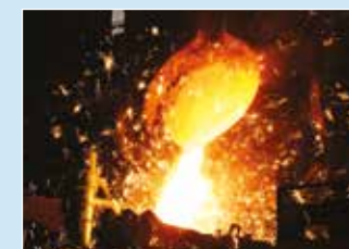
Liquid metal chemical correction in induction furnace
