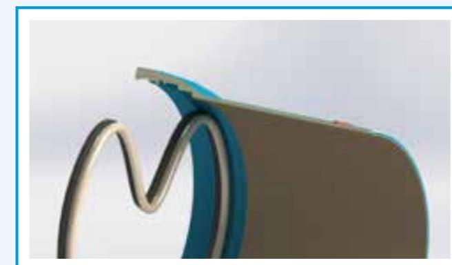
Section views of the gasket looping and seating inside the groove
