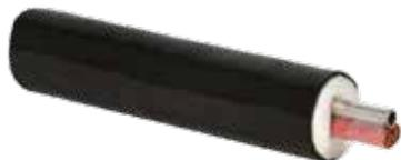
Jindal SAW's Pre-insulated and Electric Traced tubing products are used where steam is not available or steam supply could be interrupted. Depending on the application various types of pre-insulated and electric-traced tubing are available, i.e. with parallel constant wattage heating cables, with self-regulating heating cables, with power limiting heating cables, with series heating cables, etc.
